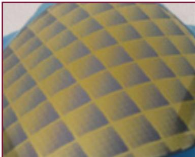
Si: diameter: 3 in to 200 mm; thickness: 50–725  $\mu\text{m}$
