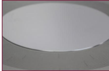
Si carriers: diameter: 2 in to 200 mm; thickness: 280–725  $\mu\text{m}$
